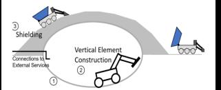
USMC Printed Vehicle Hide 3D-printed and assembled vehicle hide constructed by ICON for the USMC.
